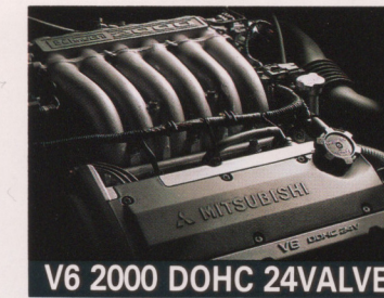
V6 2000 DOHC 24VALVE MAX.OUTPUT 170PS/7000rpm MAX.TORQUE 19.0kg・m/4000rpm
